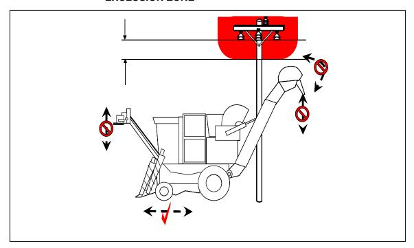
If the harvester height remains constant and cannot affect the distance between the harvester and the electric line, it is classed as a 'VEHICLE' and a safety observer is not obligatory and the exclusion zone for a 'VEHICLE' will apply. However if the profile of the vehicle changes during operation in such a way to affect the exclusion zone distance, the vehicle becomes 'OPERATING PLANT', eg if the discharge elevator of the harvester is moved up or down or alters it's discharge direction.
