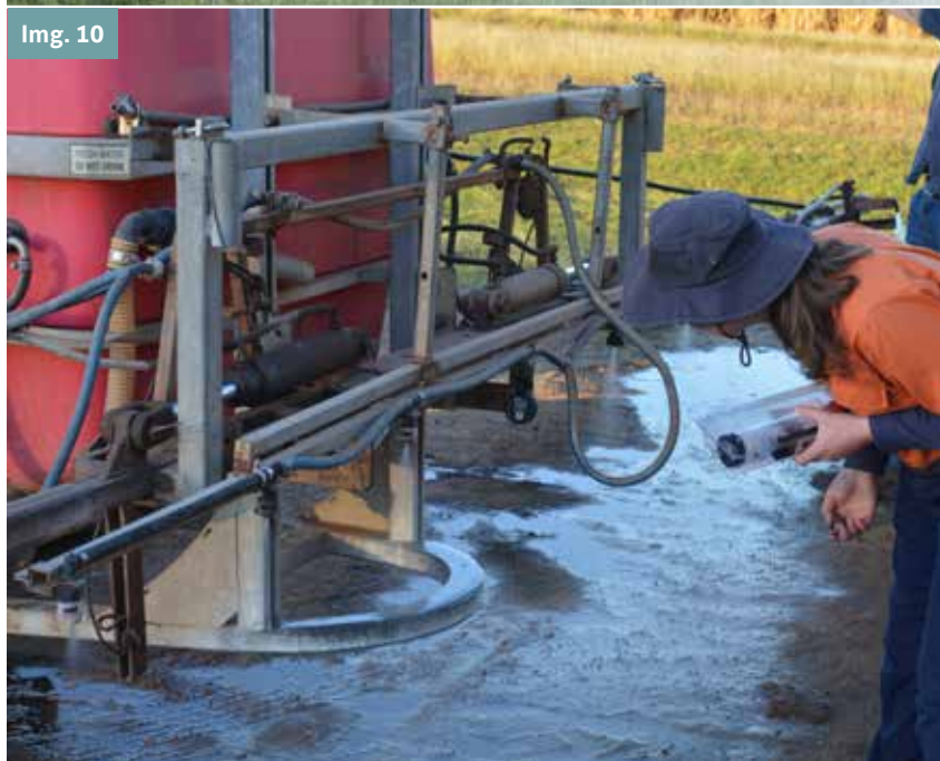
Image 9: Correct nozzle, pressure selection and adjuvant is critical to minimise drift as shown with the three left nozzles on the boom. (Photo supplied by Nufarm Australia). Image 10: Calibrating spray equipment is essential. Ensure tanks and circuits are thoroughly flushed.
