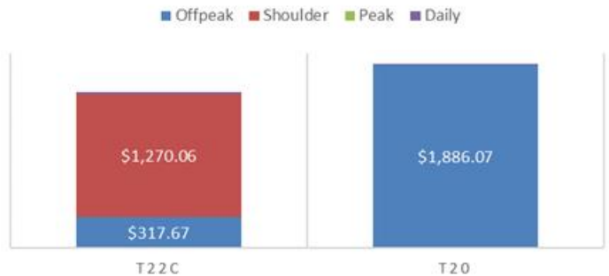
45KW MOTOR PUMPING 18 HOURS A DAY FOR 7 DAYS
